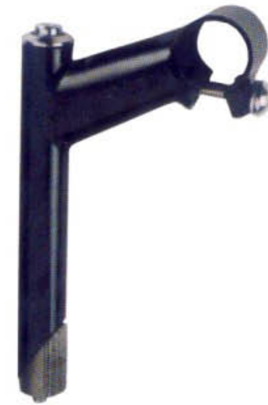
GHSS-603 STEEL HANDLE STEM Sheet thk : 1.4mm Length : 150/180mm Extension : 60-100mm Diameter : 21.2mm/22.2mm/25.4mm Finish : CP or ED
