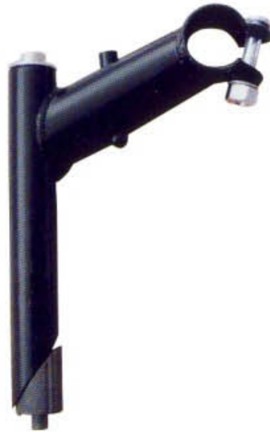
GHSS-602 STEEL HANDLE STEM Sheet thk : 1.4mm Length : 150/180mm Extension : 60-100mm Diameter : 21.2mm/22.2mm/25.4mm Finish : CP or ED
