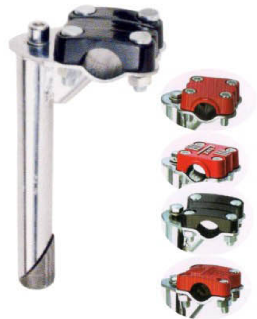
GHSS-613 STEEL HANDLE STEM BMX WITH ALLOY TOP Sheet thk : 1.4mm Length : 150-180mm Diameter : 21.1mm/22.2mm Finish : CP or ED
