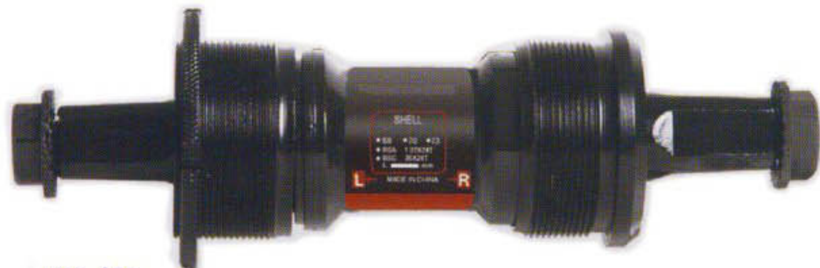
GKL-08B BB Cartridge with ball bearings 1/4"x9 Thread : 1.37x24TPI L/R & M36X24TPI R/R Available in material Cr Mo & 10B21, Available in BNCP/ED, cotterless spindle
