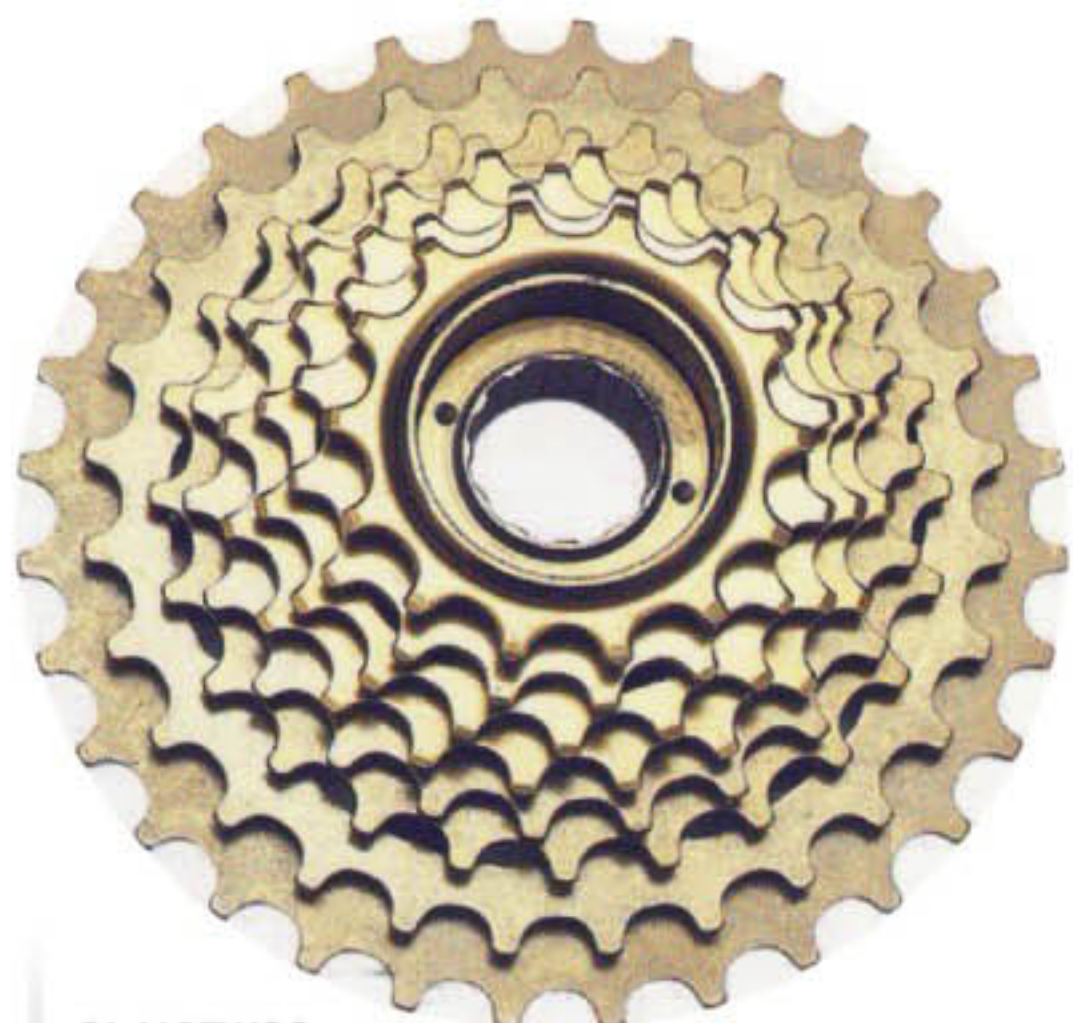
GI-MSFW28 FREEWHEEL Freewheel 8 Speed Friction Finish : Brown/ Black/ CP
