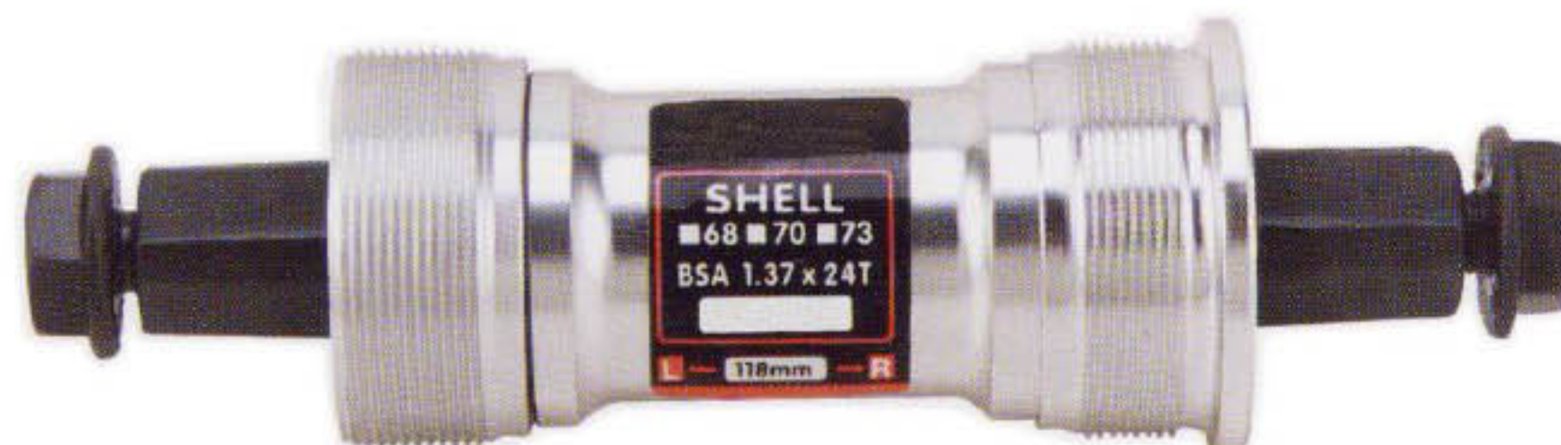
GKL-09A Cr-Mo Cotterless Spindle with alloy body 2 pcs, 2 pcs sealed bearings 16x31x10, Thread size : 1.37"X24 L/R , Finish: Black spindle, CP cups
