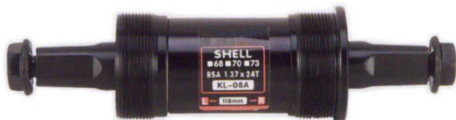
GKL-08A BB Cartridge with sealed bearings Thread : 1.37x24TPI L/R & M36X24TPI R/R Bearing size : 16x31x10 Available in material Cr Mo & 10B21, Available in BNCP/ED, cotterless spindle
