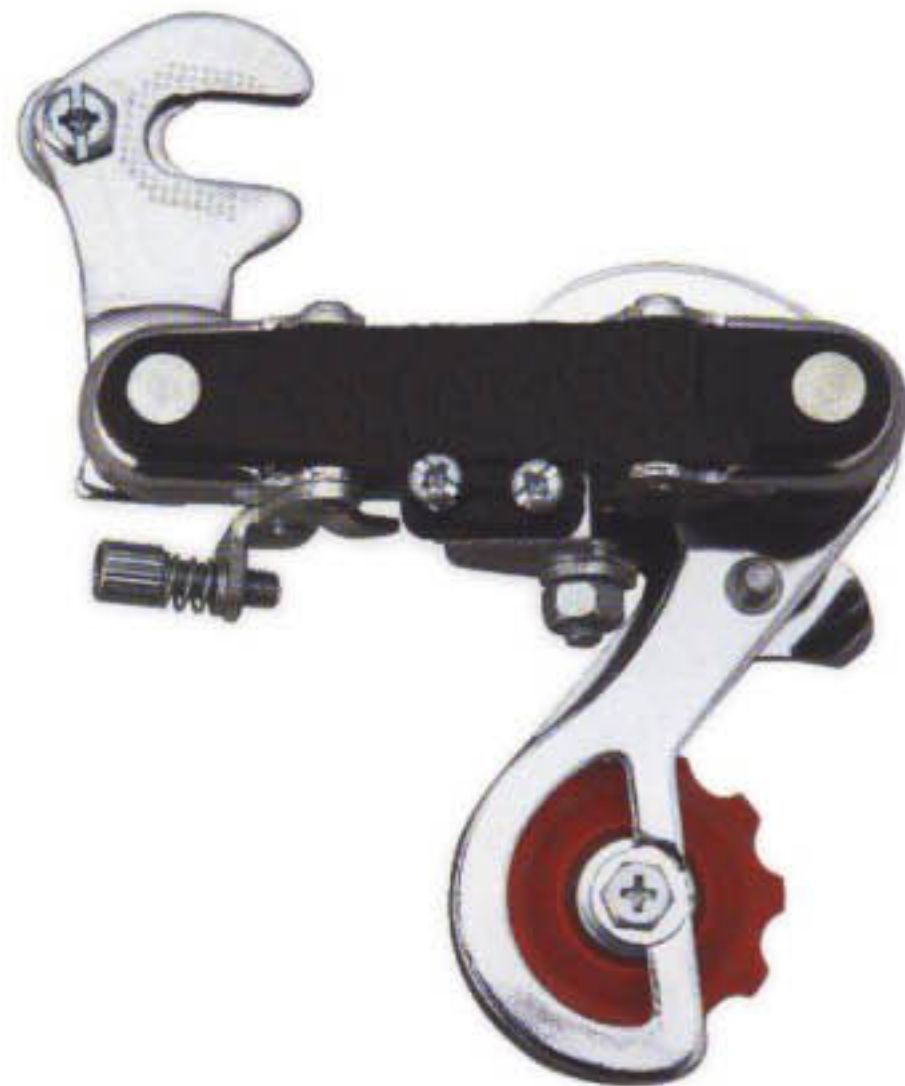
GRD-XC-03 REAR DERAILLEUR FRICTION Long Cage With Bracket. Capacity 36T Finish : CP, UCP or ED
