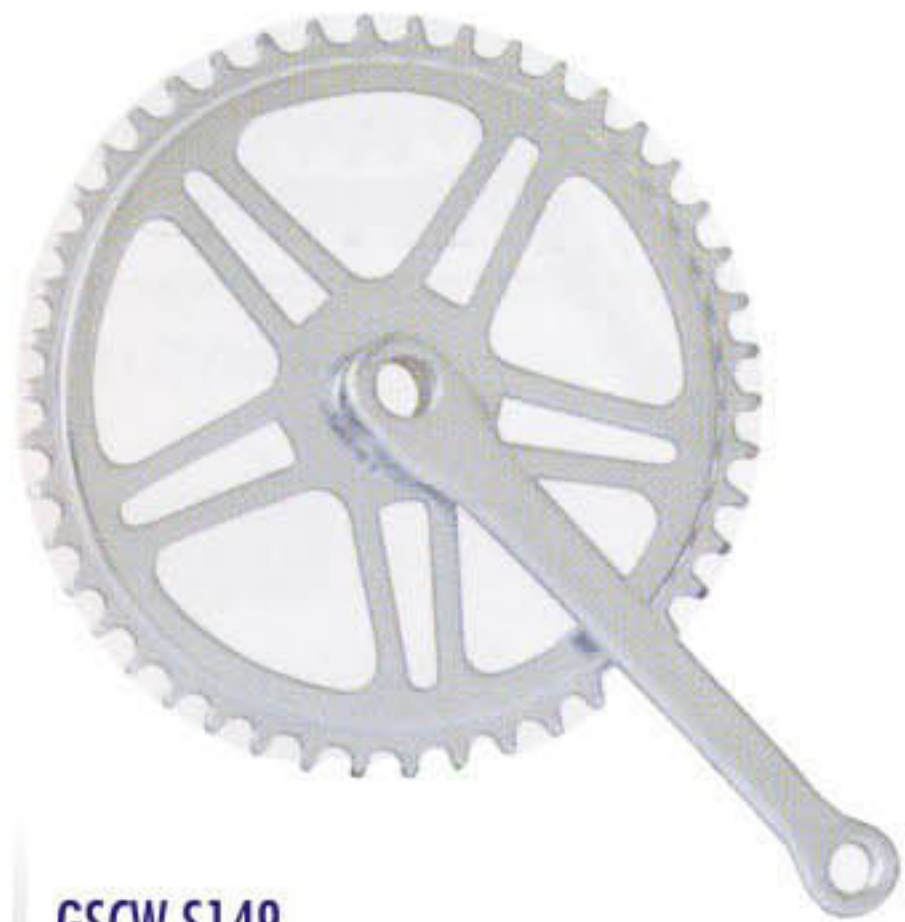
GSCW-S149 CHAINWHEEL & CRANK STEEL Italian Type. Cottered/ Cotterless Size : 28/36/40/44/48/52 Finish : CP or ED
