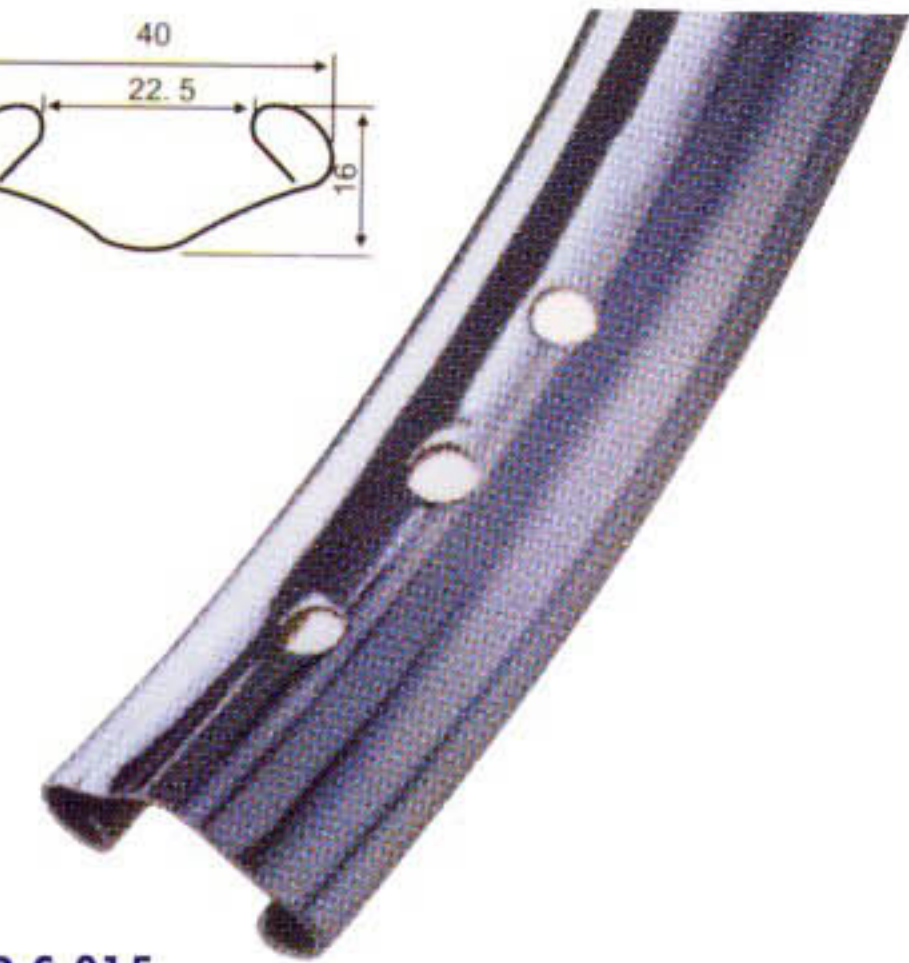
GR-S-015 STEEL RIM Sizes : 20"-28" x 1-1/2 (422-650 x 22.5mm) Spoke Holes : 16H/36H Finish : CP or ED
