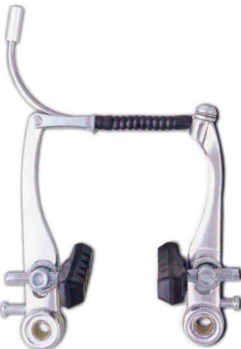
GBA-V05 V-BRAKE DESC : V-Brake alloy. Arm Length 110mm Finish : Silver/ Colors
