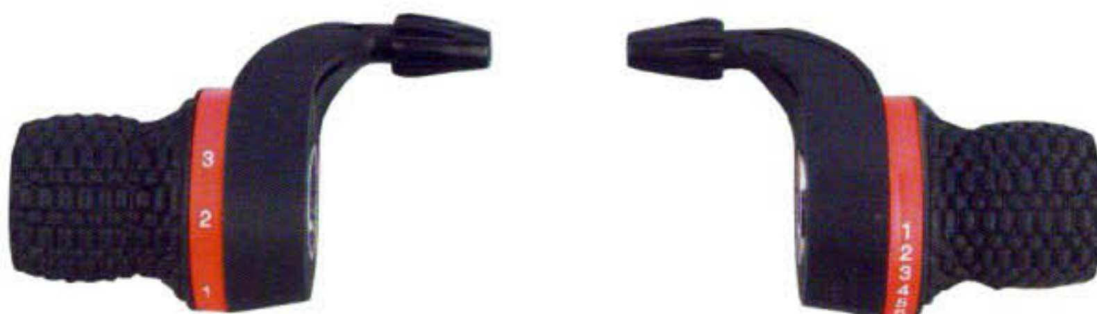
GGs-XC-3S/7S-R 21 SPEED DUAL INDEX GRIP SHIFTER Clamp dia 22.2mm Finish : na
